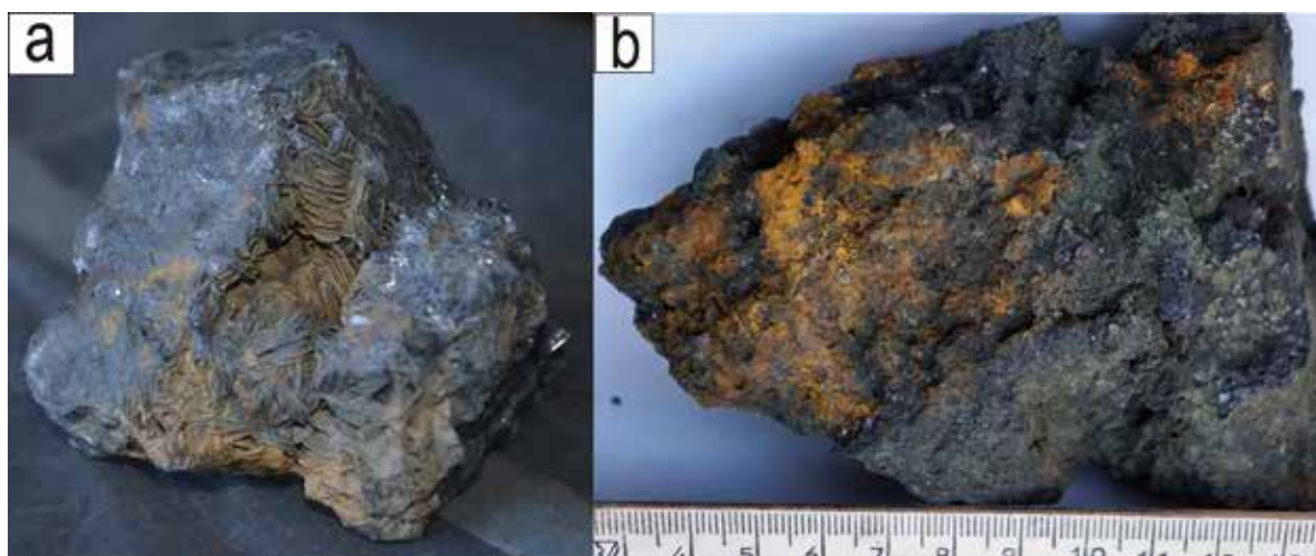
Figure 3. Samples collected from the Beck waste rocks: a) “mushketovite” pseudomorphs of magnetite after hematite; b) iron-oxides and hydroxides in skarn.
