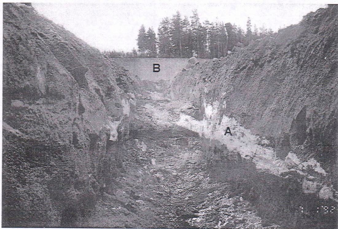
Figure 4. Horonpää gravel pit. Interstadial diatomite layer (A) and the strata (landscaped) overlying it (B) (cf. Fig. 3). Photograph: K. Nenonen.
