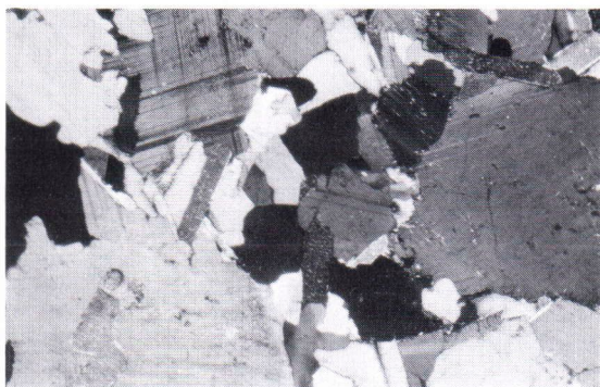
Fig. 7. Photomicrograph. Homogeneous granite-like rock (tonalitic). No signs of schistosity. Plagioclase, quartz, biotite. 40 X, + nicols.
