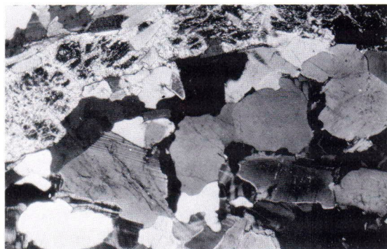
Fig. 5. Photomicrograph. Gneiss from the northeastern point. Quartz, plagioclase, microcline, biotite and aggregate of fine-grained mica, probably pseudomorph of cordierite. 40 X, + nicols.
