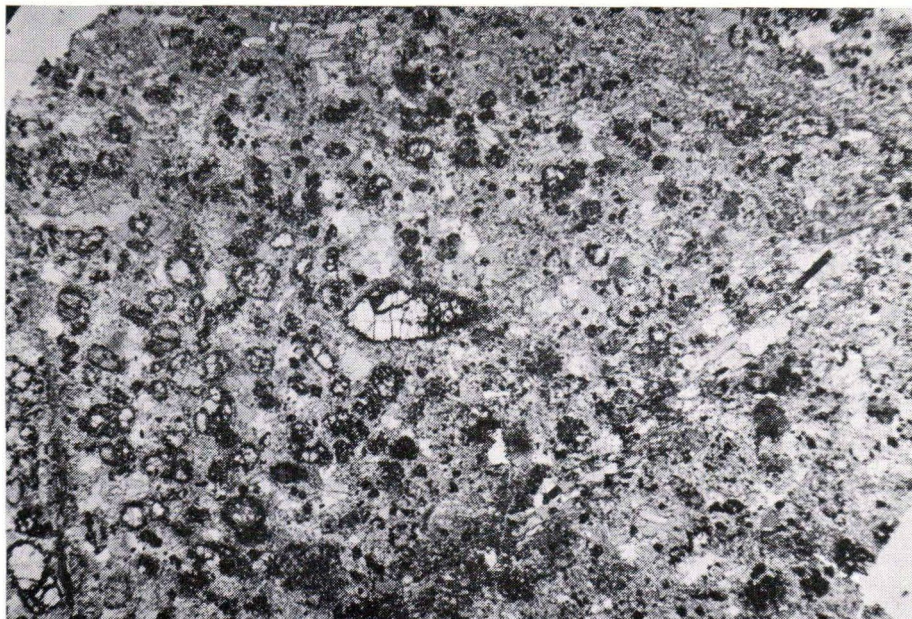
Fig. 3. A. Porphyritic dyke with fresh olivine phenocrysts, rimmed and fracture-filled by magnetite. DH 2/192.2.
