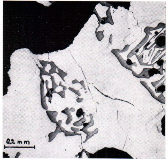
Fig. 4 Ilmenite (dark grey) partly replaced by chalcopyrite (white). Slightly harder pyrrhotite grains (white) within the chalcopyrite.
