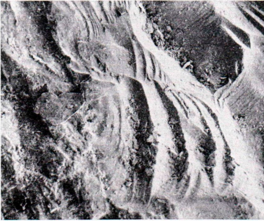
Fig. 8. Sample c (magn. 500 ×). This is a micrograph illustrating the conchoidal breakage patterns presented by a glacial grain. The variety in size of the conchoidal fractures is characteristic of glacial grains. The right side of the photograph displays a rather fresh surface because this portion is situated within a depression but the surface becomes rougher towards the left where it is less protected. This roughness is due to the presence of upturned plates. Note that there is also roughness and mechanical breakage on the protruding portions of the conchoidal fractures. The upturned plates as well as the roughness and mechanical breakage on the protruding portions are probably the result of colian transport.
