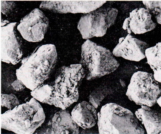
Fig. 10. Sample b (magn. 250 ×). The micrograph shows a group of grains belonging to the fine fractions (< 0.2 mm). The grains have a distinct faceted appearance very similar to that of photographed loess particles. (Compare with Smalley and Taylor 1970, p. 30 and with Krinsley and Doornkamp 1973, pp. 51–52). Adhering particles are also present as in the loess photographs.
