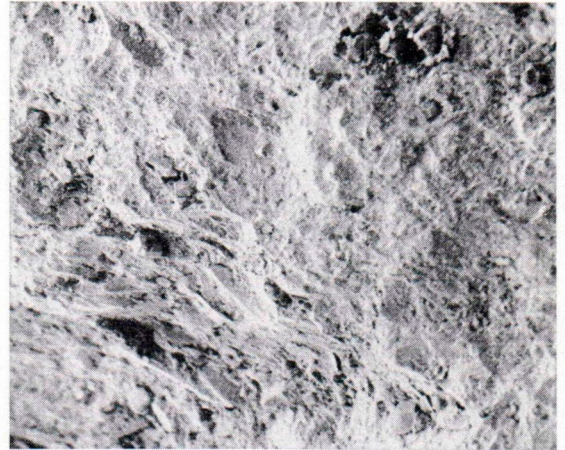
Fig. 7. Sample b (magn. 1000 \times ). This is a close-up of the surface of an eolian grain completely covered with upturned plates. Upturned plates are characteristic of eolian environments and they probably cause the frosty appearance under the binocular microscope.
