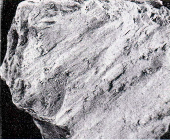
Fig. 4. Sample a (magn. 250 \times ). This micrograph shows a fairly flat striated surface on a sub-rounded grain (No. 12 of Pettijohn's scale). The striations are probably due to mechanically broken cleavage planes which were broken when a portion or portions of the grain were separated off, possibly during glacial grinding. Conchoidal breakage patterns can be seen at the upper right corner of the picture at the edge of the striated surface. The conchoidal fractures grade into upturned plates, but these are hardly visible in the photograph. The grain reflects a strong mechanical episode followed by subaqueous and eolian stages. The criteria for subaqueous environment have been V-shaped marks and blocky conchoidal fractures, for eolization upturned plates.
