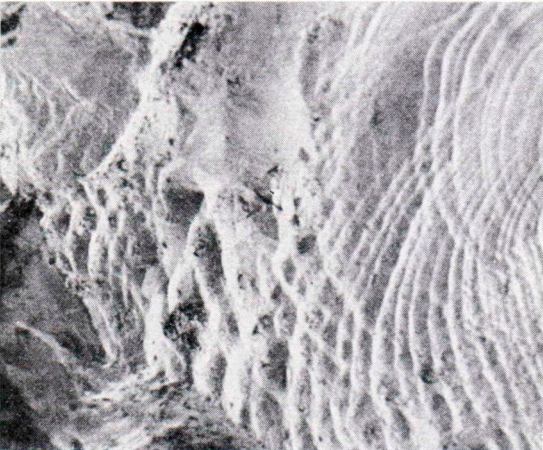
Fig. 6. Sample b (magn. 300 \times ). This grain presents a rather large surface covered with conchoidal breakage patterns. The photographed area is almost dominated by two fractures spreading from the right and which are probably the result of two different impacts. The high relief and conchoidal patterns are typically glacial textures. The occurrence of upturned plates on some of the edges and protruding parts of the grain hints at an eolian episode, but its influence on this grain is rather poor.
