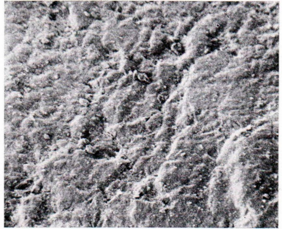
Fig. 9. Sample c (magn. 2000 ×). As in Fig. 7, this micrograph shows again upturned cleavage plates on a colian grain. The apparently subdued topography is due to incorrect focusing.
