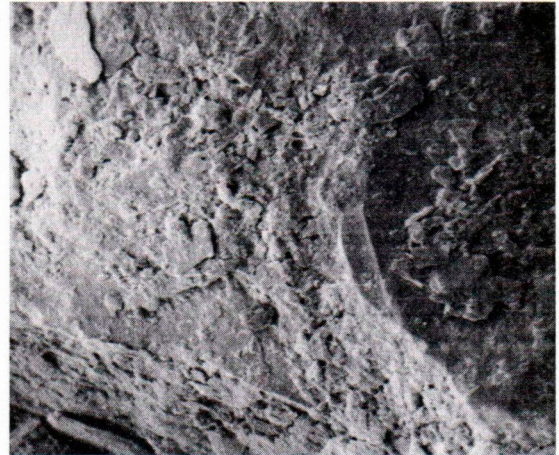
Fig. 11. Sample c (magn. 2500 ×). This is a close-up of one of the grains in Fig. 10. The rather smooth surfaces almost devoid of conchoidal patterns suggest that the facets are due to mechanical breakage along cleavage planes. Upturned plates occur, but they are never as common as in the larger-sized grains. This seems to indicate that the finer-sized grains did not undergo as much saltation as their larger counterparts.
