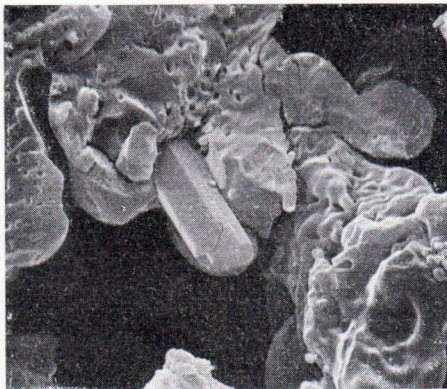
FIG. 5. Two intergrown crystals of an unknown mineral developed in a cavity of nickelhexahydrite. (1650X).
