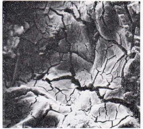
FIG. 2. Rather smooth surface of nickelhexahydrite. Fine cracks may have developed due to dehydration. (1120X).
