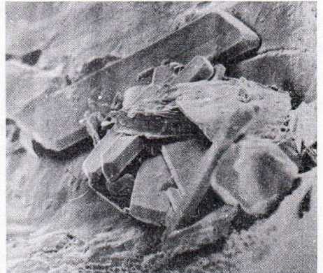
FIG. 6. Crystals of the unknown mineral, each bounded by very regularly shaped faces, occur on the rather smooth surface of nickelhexahydrite. (2400X).
