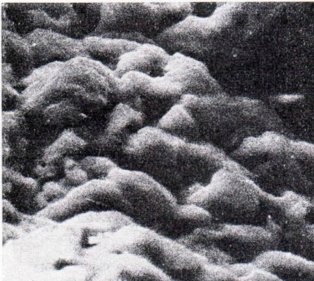
FIG. 3. Very irregular »knobby» nickelhexahydrite surface. (3700X).
