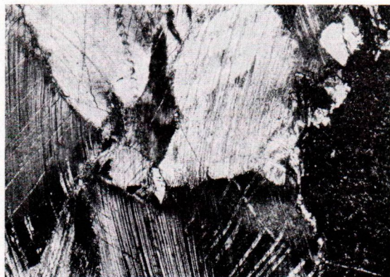
Fig. 3 A. Microphotograph of the contact between crystalline limestone and trapp diabase.
