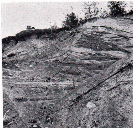
Fig. 3. A view from the same gravel pit at site No. 2 as in FIG. 1. The arrows point to weathered limestones. The numbers 13–16 refer to the soil samples analyzed and plotted in Table 1. Also marked in the figure are the heights in meters above sea level.
