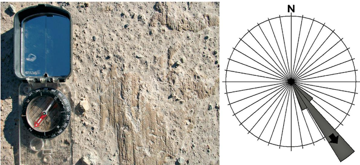
Fig. 7. Glacial striations on dolomite surface in Turkalne quarry and orientation of striations by StereoNet plot (number of measured striations is 55 and the mean azimuth is  $143^\circ$ , lower hemisphere projection).
