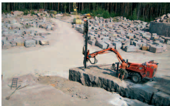
Figure 5. Ladozhskoe deposit on the Karelian Isthmus (Leningrad region). Splitting of primary monolith for secondary monoliths for commercial blocks production.
