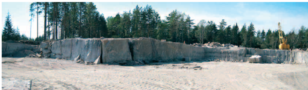
Figure 3. Ladozhskoe deposit on the Karelian Isthmus (Leningrad region). Quarry for granite block extraction.
