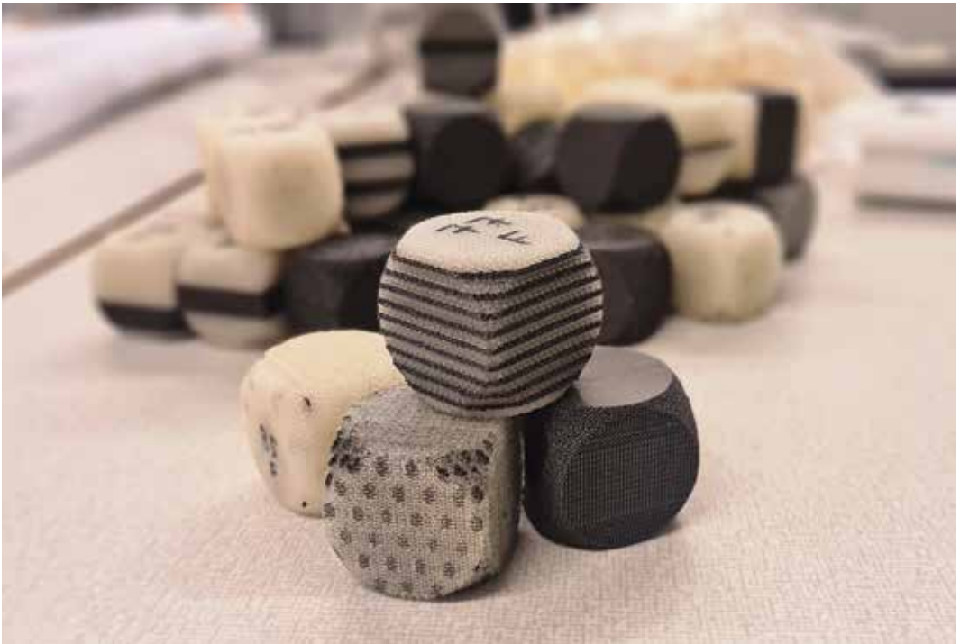
Figure 4. 3D printed synthetic “rocks” with varying graphite content and distributions. Photo: Ana Haivio Reales.
