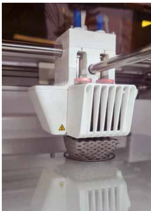
Figure 1. Fused filament fabrication 3D printer constructing a synthetic rock sample layer by layer at the research laboratory in GTK, Espoo. Photo: Ana Haivio Reales.
