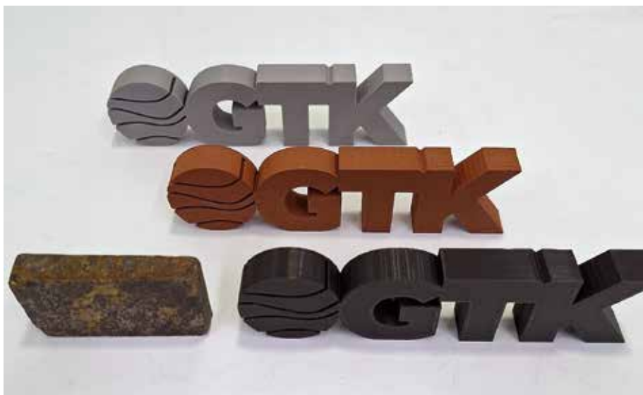
Figure 2. GTK logos 3D printed using different processing stages of copper ore from Outokumpu with PLA bioplastic binder as material: ground, unseparated ore (front), beneficiated copper (middle), and tailings waste material (back). Outokumpu copper ore sample on the left. Photo: Heli Lallukka, GTK.
