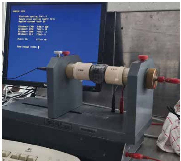
Figure 5. Measuring the electrical properties of graphite-rich 3D printed sample using the MAFRIP instrument at the geophysical laboratory at GTK, Espoo. Photo: Ana Haivio Reales.
