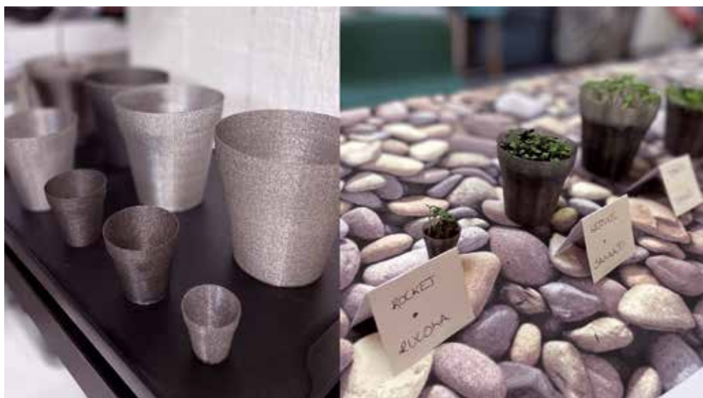
Figure 3. Left: Plant pots printed with PLA bioplastic and volcanic ash from the 2021 La Palma eruption, used as an analogue for lunar regolith (Moon ‘soil’) in In Situ Resource Utilisation (ISRU) project. Right: Growth experiment in ISRU project using varying soil and volcanic ash ratios (ISRU analogue experiment). Photos: Kati Kiviniemi, GTK.
