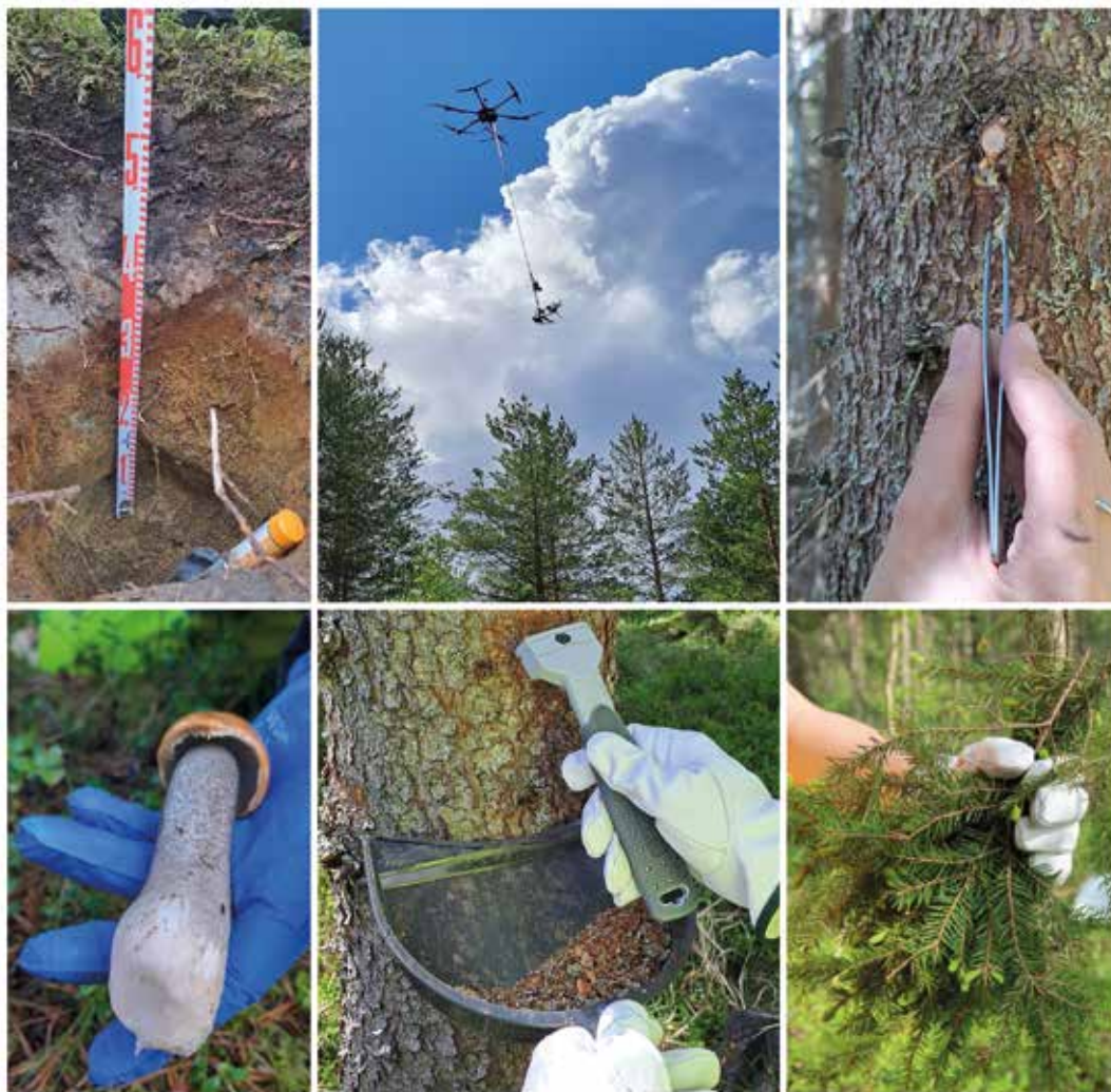
Figure 2. In DeepBEAT project, till and biogeochemical sample material is tested to discover suitability for detection of the deep-seated Saramäki VMS deposit. Upper canopy samples are acquired with a sampling device carried by the drone. Photos: Sari Romppanen and Maarit Middleton.
