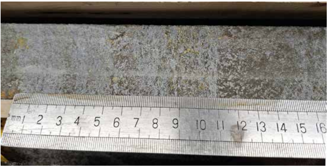
Figure 1. Typical sample from the Saramäki deposit hosted by biotite- and quartz-rich tremolite skarn rock. Main ore minerals include pyrrhotite, chalcopyrite, and sphalerite. Photo: Tuulia Häkkinen.
