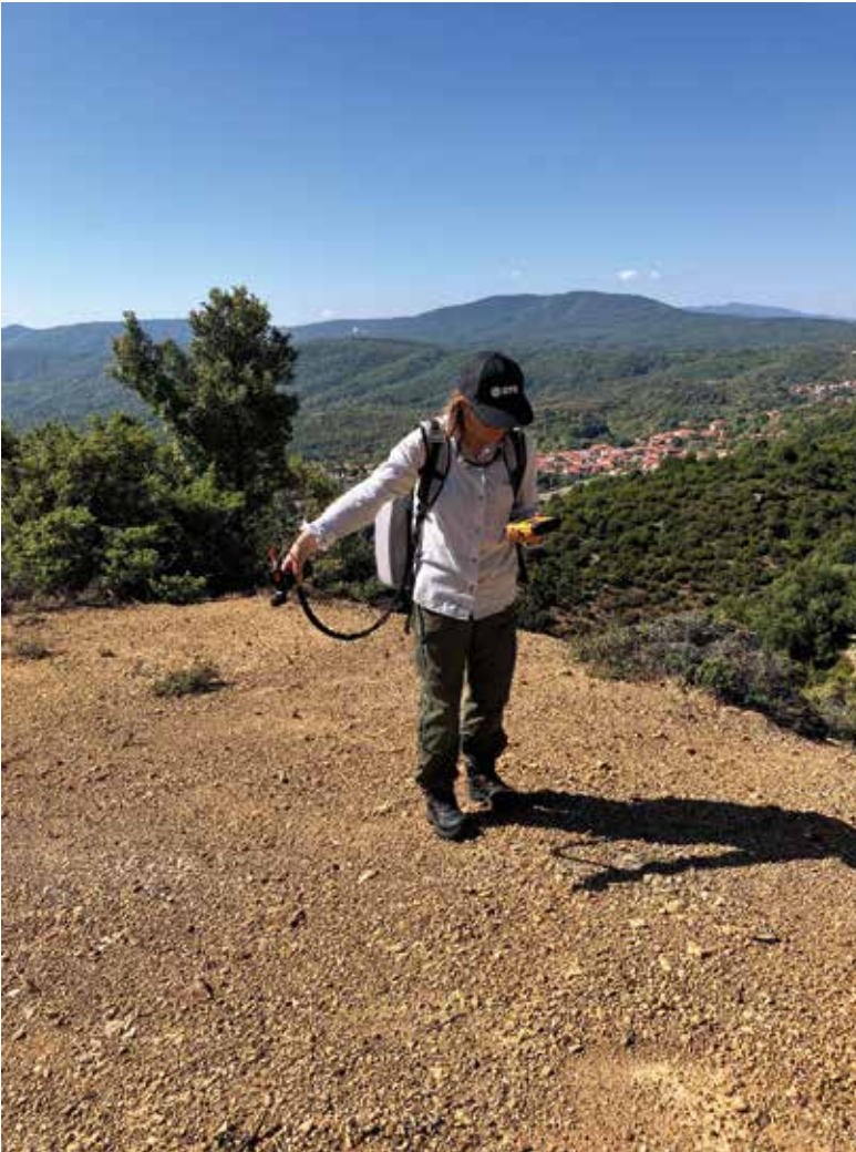
Figure 1. Spectral data acquisition using a field spectrometer. Photo: Martin Schodlok.
