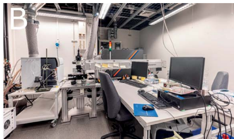
Figure 2. Metrohm ECO tandem ion chromatograph used for analysis of major ionic components of water samples (A) and Agilent 7900 ICP-MS instrument combined to coherent 193 nm laser (GeoLas MV) used for microanalysis (LA-ICP-MS) of solid materials (B).
