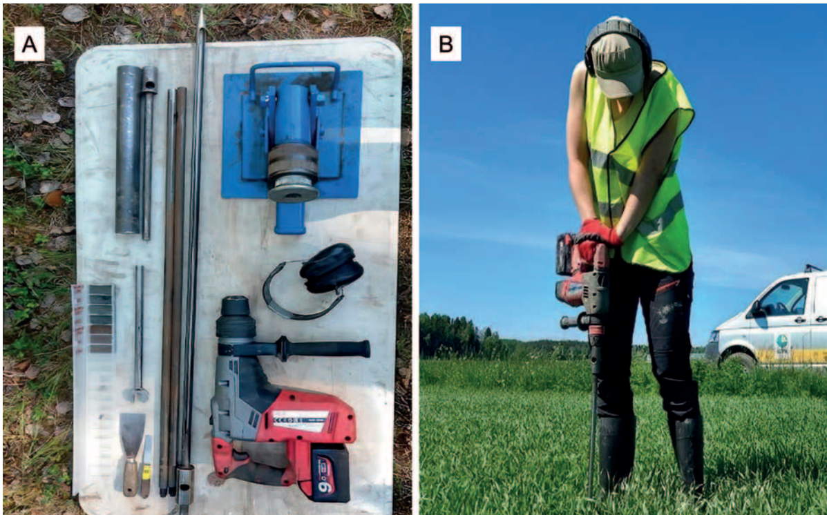
Figure 6. Percussion drill and samplers (A) in operation (B). Photos: GTK / Krister Dalhem.
