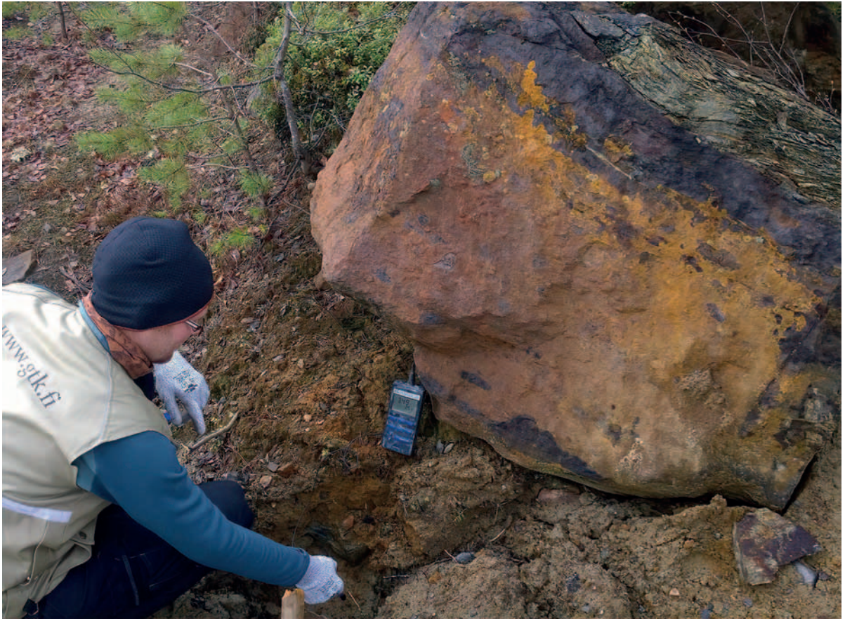
Figure 11. Oxidized unsorted acid sulfate soil material with pH 3.5, containing boulders and fragments of black shale, in this case transported only a short distance. Photo: GTK / Stefan Mattbäck.
