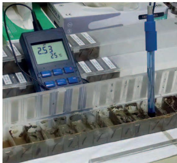
Figure 7. Sample container (chip-tray) used for incubation of collected samples. The pH is measured by inserting the pH-electrode directly into the moistened sample. Photo: GTK/ Hannu Hirvasniemi.
