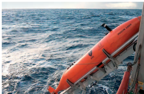
Figure, left: Carbonate crust slabs on the seafloor, overgrown by sponges. Figure, right. The HUGIN AUV was used for collecting detailed sidescan sonar data and photos along sections.
