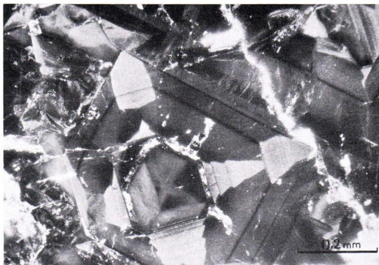
FIG. 2. Zoned cassiterite with overgrowth pyramids well developed. Polished section, oblique illumination. Specimen no. 439. Sukula, Tammela, SW Finland.
