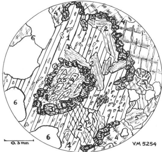
Fig. 4. Pyroxene-bearing monzonitic granite. W of Kowa. 1 = pyroxene; 2 = uralitic amphibole; 3 = epidote; 4 = microcline; 5 = plagioclase; 6 = quartz. N //.
