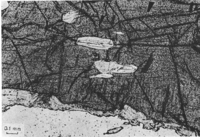
FIG. 5. Microphoto. A portion of a hypersthene grain with gedrite inclusions and a surrounding gedrite ring. 1 nic. Lake Juurikka, Toivaiskylä, Kiuruvesi.
