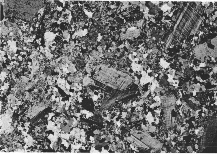
FIG. 5. Granite porphyry. Point 9 on Fig. 2. The insets are mainly microcline, to the left also consisting of plagioclase. N+, Magn. 8×. Photo: E. Halme.
