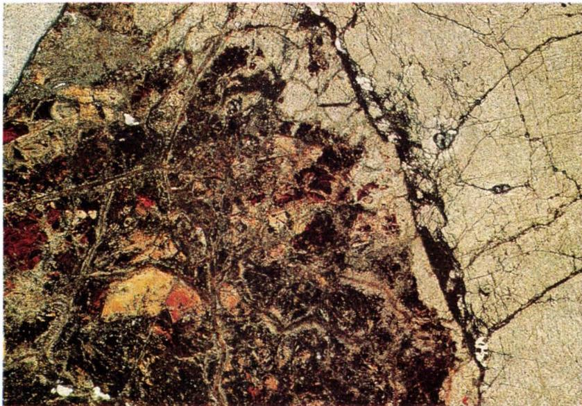
FIG. 7. Calcio-gadolinite. Right margin albite. Between the inhomogeneous metamict calcio-gadolinite and albite there is a rim of crystalline calcio-gadolinite. The narrow light rims around the fissures in calcio-gadolinite have the same optical orientation as the crystalline gadolinite mentioned above and as the large yellowish-brown homogeneous region in the middle of the crystal. Magn. 11 x. Photo: Erkki Halme.
