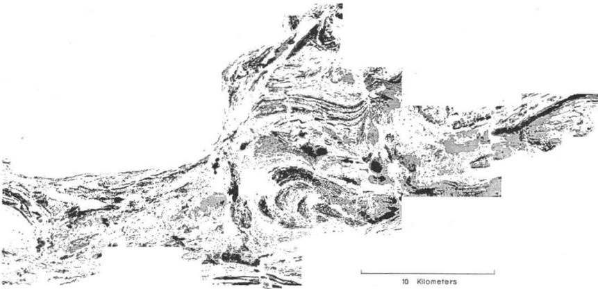
FIG. 2. Magnetic vertical intensity ( $\Delta Z$ ) in the Orijärvi region (1:400 000) based on 500 000 ground observations. Black: > 400 gammas. Shaded: 200—400 gammas. White: < 200 gammas. The round white patch in the center is not surveyed. From Tuominen 1957.
