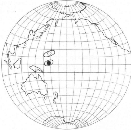
Fig. 3. Virtual magnetic pole positions and the ovals of confidence according to the measurements of the magnetic directions of the Satakunta olivine dolerites. o = pole position according to the measurements before magnetic cleaning, ● = pole position calculated after demagnetization.
