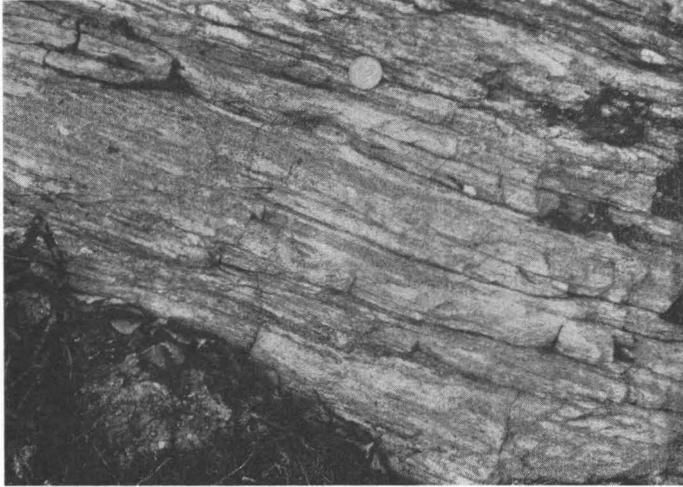
Fig. 22. Gneiss from western margin of conglomerate at Kukkomäki. In the upper part of picture, facing east, there occurs augen gneiss with the appearance of a conglomerate. Kukkomäki, Vieremä.
