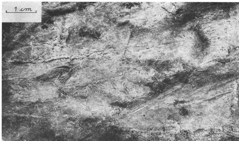
Fig. 9. Hornblende porphyroblasts in the biotite-epidote-plagioclase schist. Around the porphyroblasts is a light gray halo. Metelinmäki, Salahmi, Vieremä.
