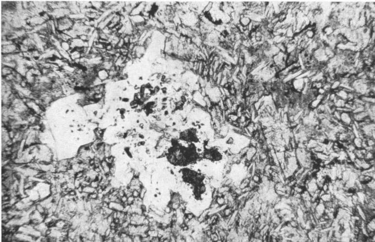
Fig. 2. Resorbed aggregate of plagioclase in the basalt. Dark grains in the plagioclase are reddish spinel. Asuk, Disko. Thin section. One nic. 100 ×.
