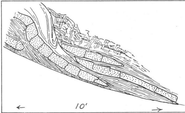
Fig. 9. Telescoped sandstone beds with tension joints which may lead to boudinage. A larger thrust begins to form and shale is crenulated next to it. Total effect about 3 meters.
