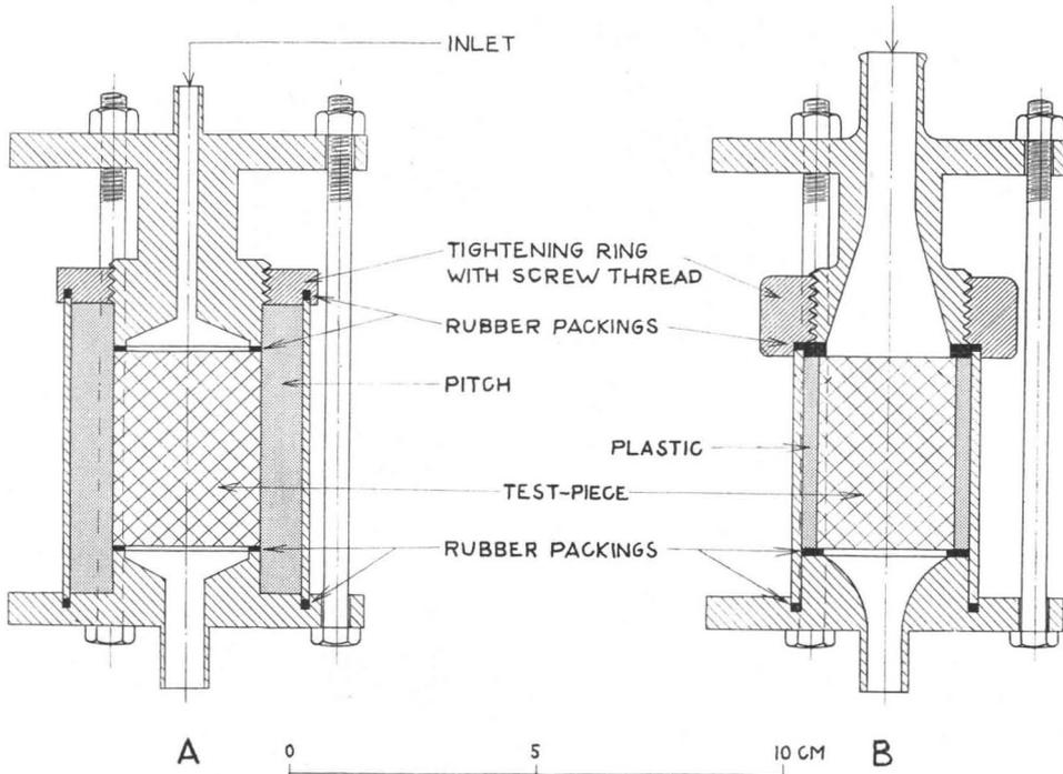
Fig. 2. Apparatuses used for the determination of the rate of dissolution of Alnö dikes.
