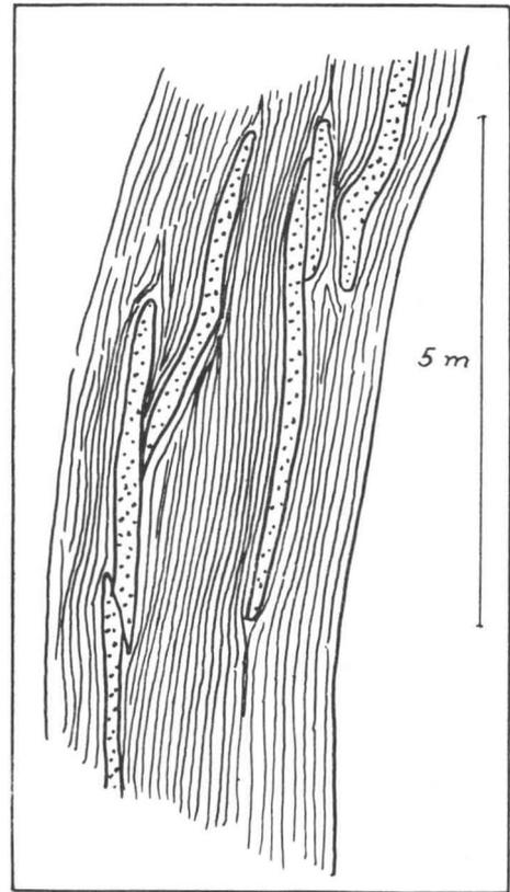
Fig. 8B. Telescoping in 2 beds by about equal amounts.
