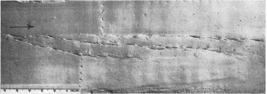
Fig. 17. Wedges in experiment with 3 layers of soft clay. Displacement is indicated by vertical rows of dots above right end of scale.
