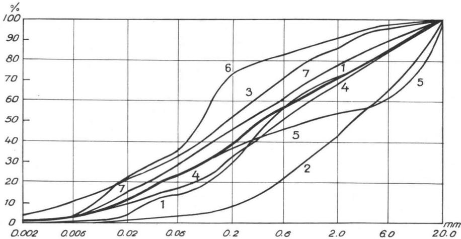
Fig. 7. Cumulative curves for the till in the Hämeenlinna region. The thick line represents the average mechanical composition of approximately fifty till samples. 1 = Salpausselkä till, Turenki, 2 = material of a small end moraine, Renko, 3 = fine sandy till, Tervakoski, 4 = material of a small end moraine, Lastujärvi, 5 = gravelly till, Hämeenlinna, 6 = fine sandy till, Rehakka, 7 = sandy till, Vähikkälä.
