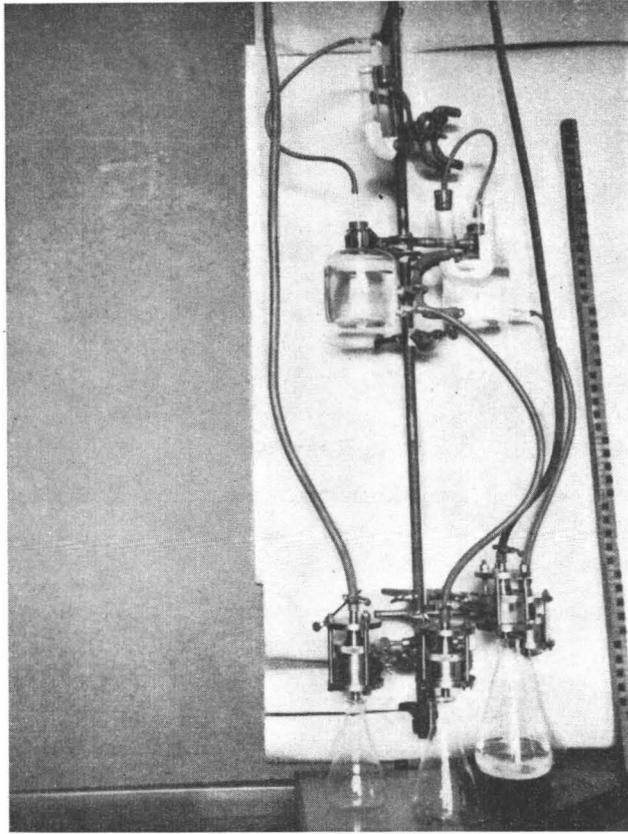
Fig. 3. Assemblage of apparatuses used for the determination of the dissolution ratio of the kimberlitic dikes. Two apparatuses are put under 0.5 and two under 1.0 metres water pressure. Two of the U-shaped vessels absorbing the  $\text{CO}_2$  of the air are seen. During the experimental run the beakers which collect the percolating water were placed in a freezing-mixture.
