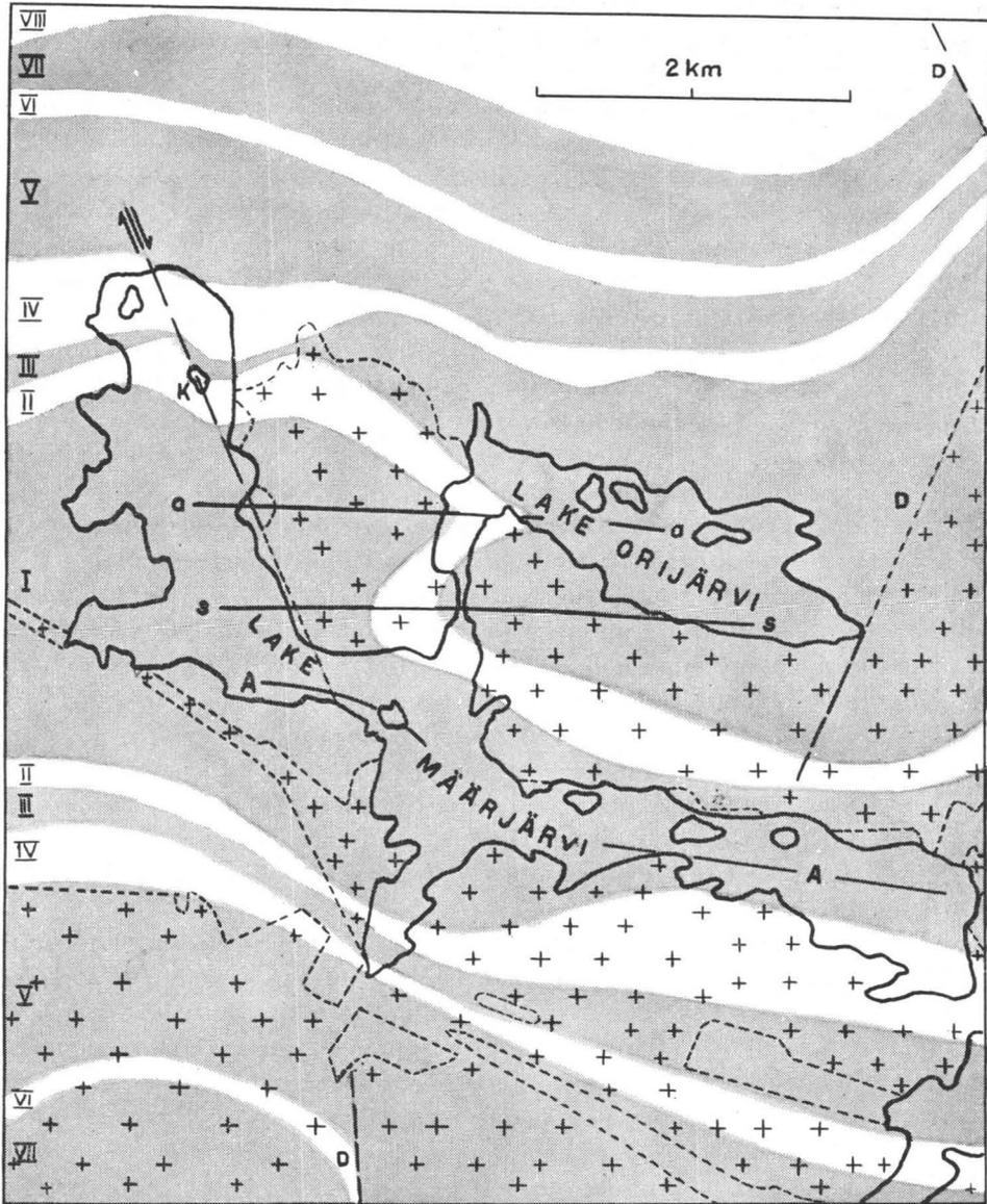
Fig. 2. Map of the Orijärvi granodiorite and surroundings. Crossed areas are granodiorite. A—A = Määrjärvi anticline. a—a = secondary anticline. s—s = secondary syncline. D = downthrown side of thrust fault. Arrows = strike-slip fault. K = Isle of Kurksaari. Shaded = zones of higher magnetic intensity. White = zones of lower magnetic intensity. Roman numbers I—VIII show the apparent sequence of strata. The magnetic zoning seen in the map is compiled from measurements at over 50 000 stations.
