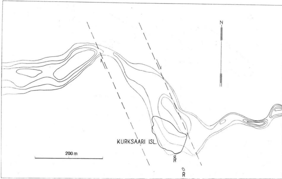
Fig. 3. Magnetic vertical intensity map revealing the Kurksaari strike-slip fault. Contours: 400, 800, 1 600 and 3 200 gammas. Dashed lines indicate the borders of the fault zone. R = small rocks.
