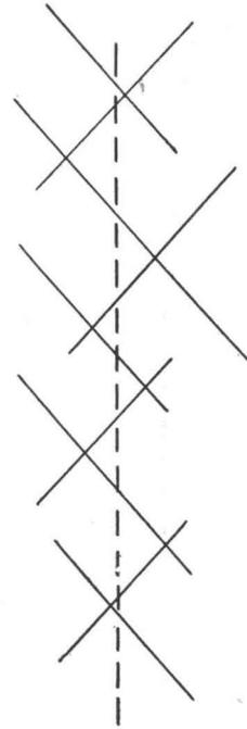
Fig. 1. Two crossing *en échelon* faults. The broken line shows the main direction of the valley formed by weathering. Schemed.
