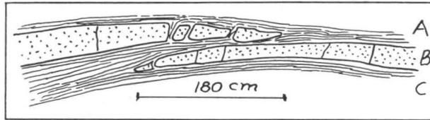
Fig. 7. Sandstone bed in shale. Wedged with boudinage in upper wedge. Devonian near Zell a. d. Mosel, Germany.
