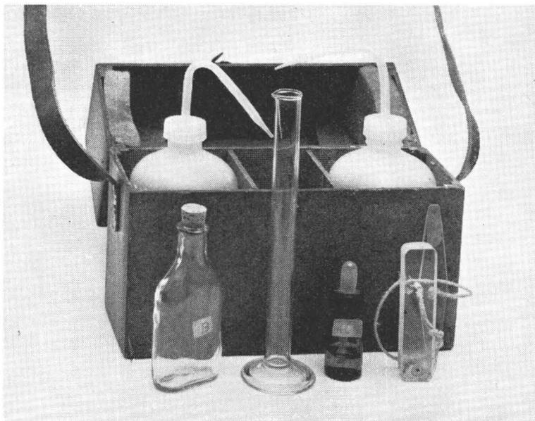
Fig. 1. Kit for field analysis. It contains: 1 measuring cylinder (25 ml), 1 plastic measuring scoop and spoon, 2 plastic squeezing bottles (one for dithizone and the other for buffer pH 8.5), 2 small bottles (for buffer pH 2.0 and KCN solution).
