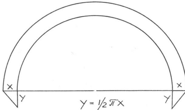
Fig. 15. Amount of displacement in a concentric fold after Busk (1929, p. 10).
