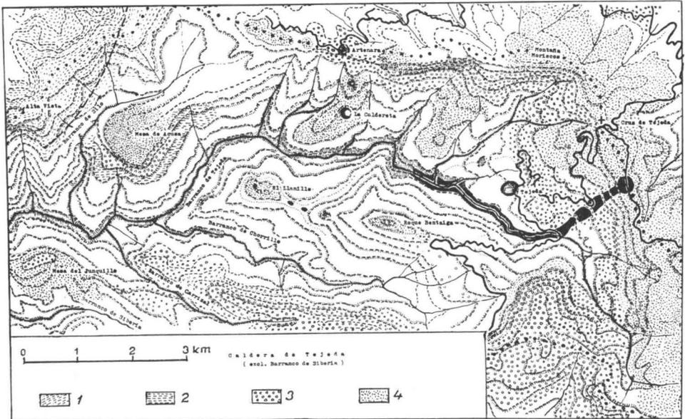
Fig. 5. Topographic-geologic map of Caldera de Tejada (excl. Barranco de Siberia). White, unmarked area inside the caldera: old trachytes, dislocated. 1 = trachytes in Alta Vista. 2 = trachyphonolite in Mesa de Acusa. 3 = Roque Nublo agglomerate. 4 = Post-Miocene olivine basalts. Dark stream to the right: young basalt lava following Barranco de Tejada. Dotted line: watershed. Copied from the topogr. map of the island on the scale of 1: 25 000. Long direction: E—W.
