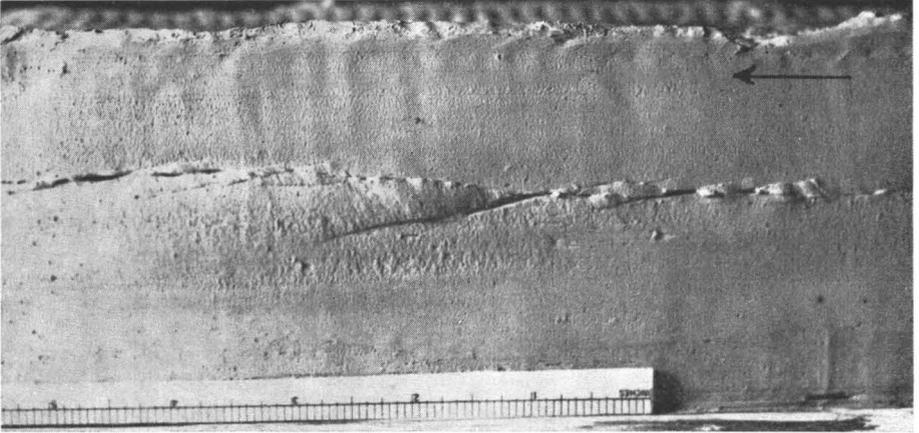
Fig. 16. Wedges in experiment with two clay layers.
