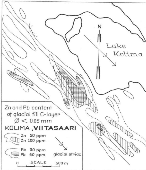
Fig. 5. Zinc and lead concentrations in soil, C layer,  $\phi < 0.05 \text{ mm}$  at Kolima.
