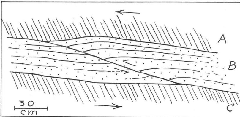
Fig. 2. Sandstone bed cut by low angle fracture with displacement of about 30 cm. Bloomsburg fm. (Silurian) Western, Md. Railroad cut opposite Great Cacapon, West Virginia.
