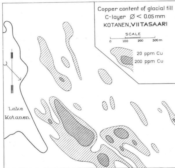
Fig. 6. Cu concentrations in till (C-layer,  $\leq 0.05\text{ mm}$  fraction) at Kotanen.
