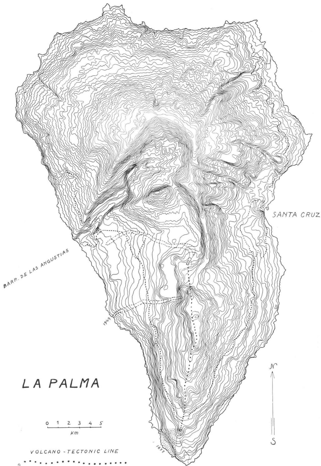
Fig. 9. Topographic map of the island of La Palma with 50 m contour interval. The dotted line represents the main volcano-tectonic fissure of the island.
