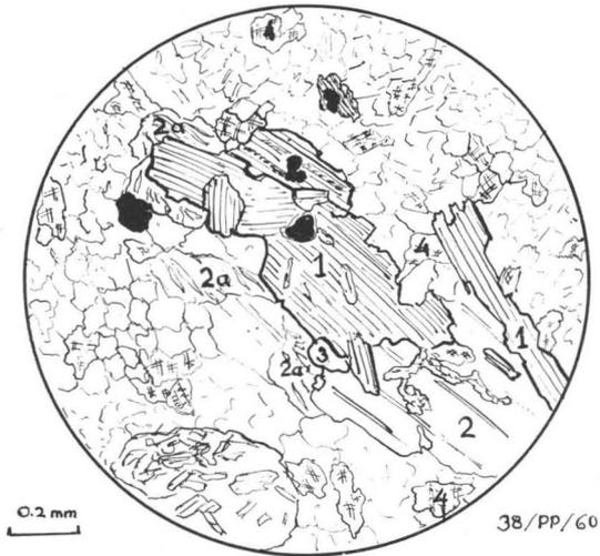
Fig. 4. Fine-grained granite porphyry on the NE. margin of the porphyrite area. A strongly muscovitized grain of plagioclase in the center of figure. 1 = muscovite, 2 = plagioclase, 2a = antiperhite, 3 = fluorite, 4 = microcline; solid black is magnetite. The matrix consists of quartz, plagioclase and microcline.
