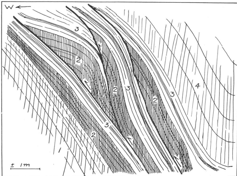
Fig. 11. Wedging in Bloomsburg shale, W. Md. R. R. opposite Great Cacapon. Shale and siltstone layers are repeated by thrusting and wedging. Anticline to left, movement essentially exaggerates bedding slip.
