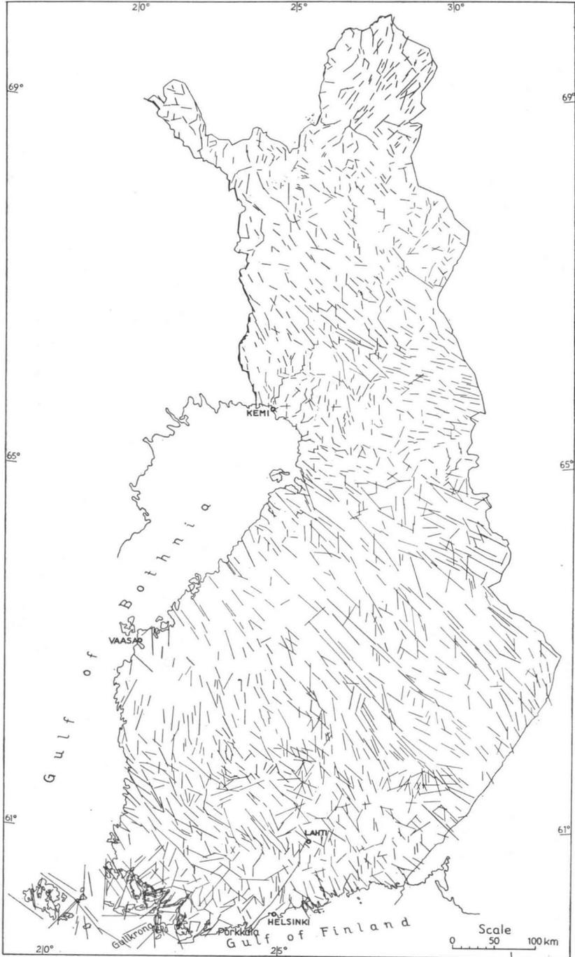
Fig. 2. The trends of the most marked fault lines in Finland.
