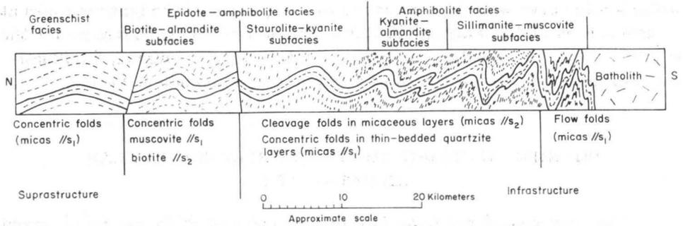
Fig. 6. Schematic section showing changes in style of folding and distribution of metamorphic facies northwest of the Idaho batholith.
