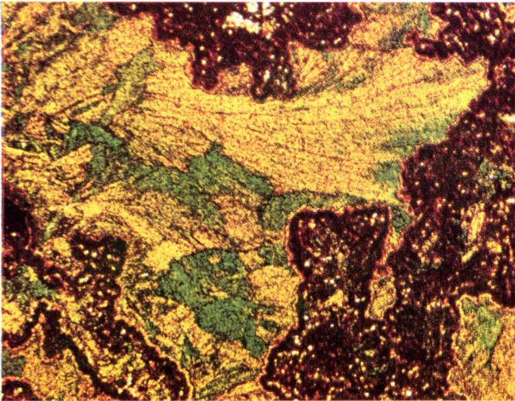
Fig. 2. Aggregates of rockbridgeite, partly altered to goethite and aluminian strengite. Without analyzer. Magn.  $77\times$ . Photo Erkki Halme.
