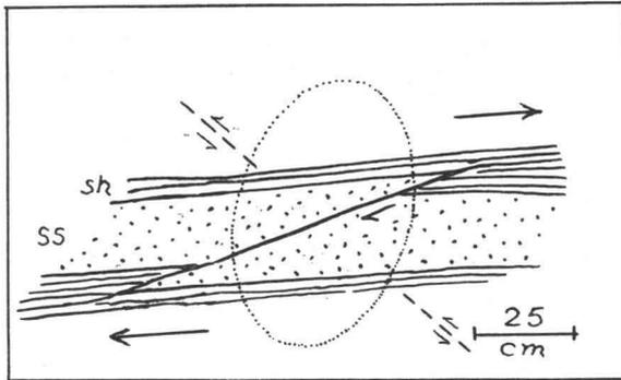
Fig. 1. Small low-angle ( $16^\circ$ ) reverse fault divides limestone bed into 2 wedges. Displacement 25 cm. Val de Fir SW Geneva (Switzerld.).
