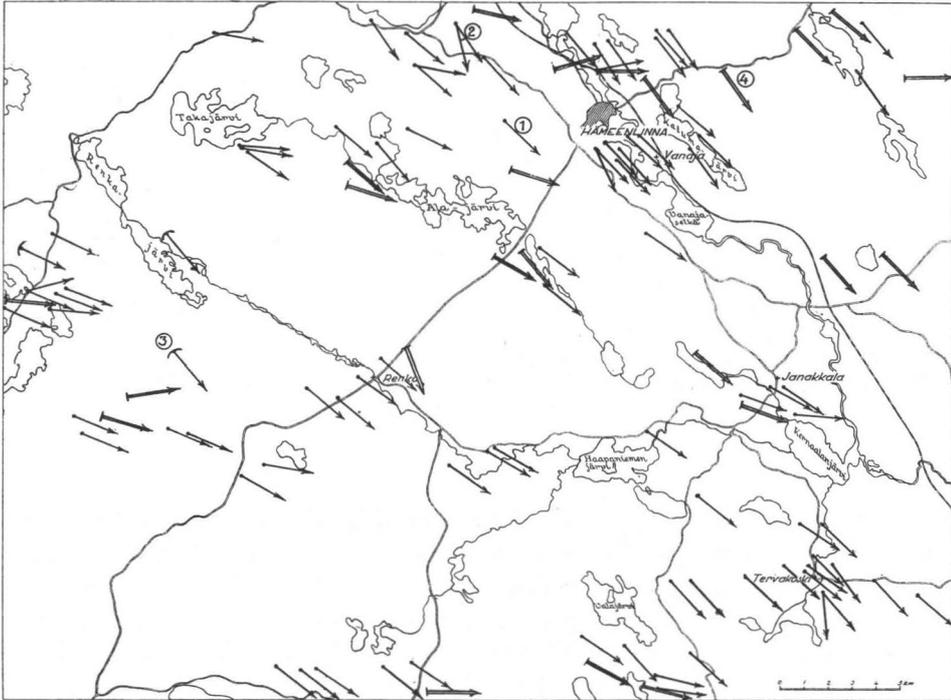
Fig. 2. The striations and till fabric in the region surveyed. 1 = trend of striations, 2 = trend of striations together with intermediate values, 3 = trend of erosion facets, 4 = preferred orientation of stones in till.
