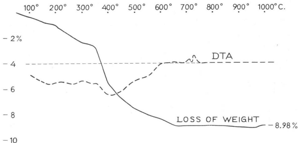
Fig. 1. Differential thermal analysis and dehydration curves of rockbridgeite.
