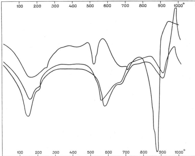
Fig. 1. Differential thermal diagrams of clays from altered kimberlitic dikes.
