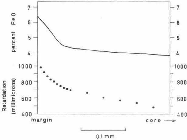
Fig. 4. Variation of optical retardation (bottom) and FeO content (top) in the zoned margin of a melilite phenocryst. Specimen VM. 362. Ipnitic block from the notch of the southern rim of the Baruta crater.
