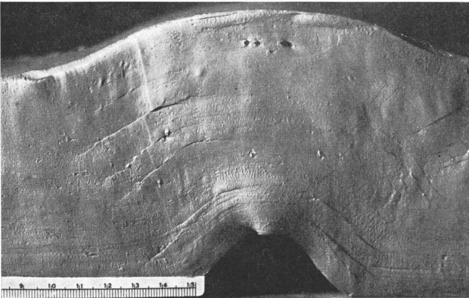
Fig. 19. »Concentric joints» (de Sitter, 1956) in clay experiment. Soon after formation of concentric joints they take the place of bedding planes and wedges form as seen in Figure 20.
