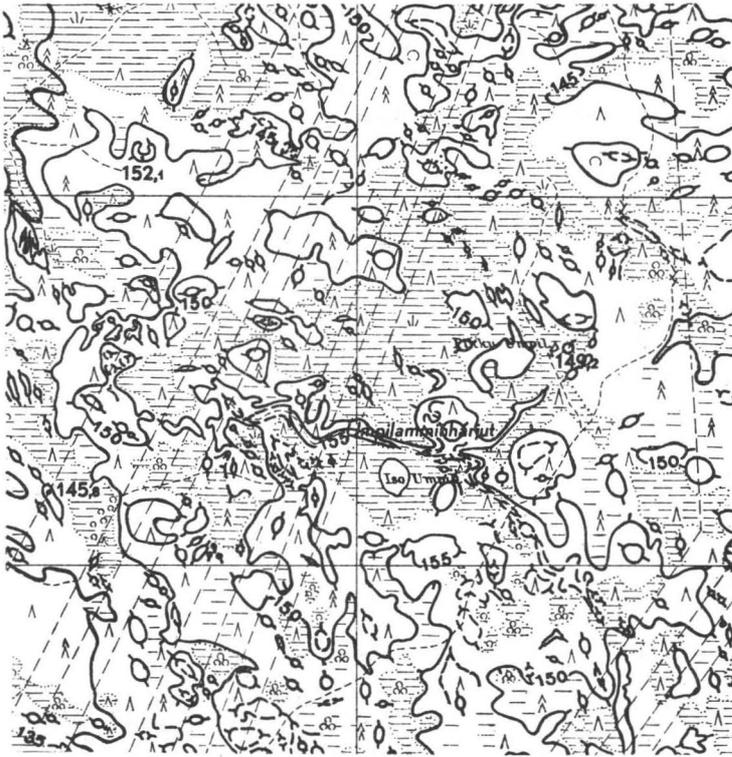
Fig. 10. A detail from the ablation moraine area located in the Vuohiniemi map sheet. The ruled lines represent bogs, the space between the elevation curves is 5 m, scale 1: 20 000.
