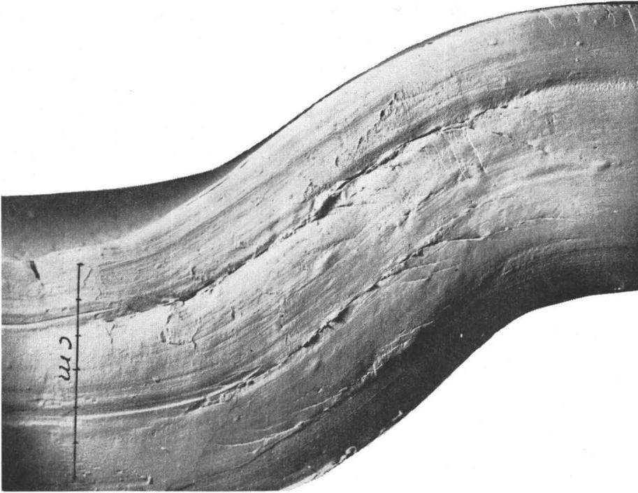
Fig. 18. Wedges in left limb of anticline with 3 layers of clay. High angle shear plane is also visible near anticlinal crest.
