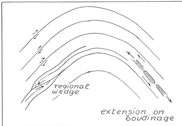
Fig. 5. Schematic fold showing boudinage (right) and wedging (left).
