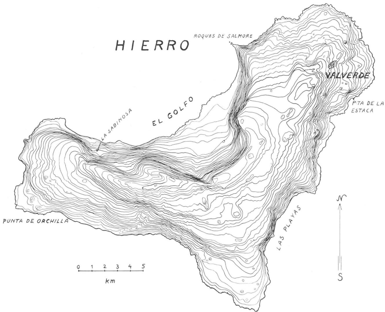
Fig. 11. Topographic map with 50 m contour intervals showing the strange outlines of the island, produced partly by fractures, partly by marine abrasion.
