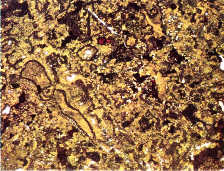
Fig. 1. Phosphatite consisting of rockbridgeite (greenish) that is partly altered to aggregates of goethite and Al-strengite (brownish), and individual grains of goethite (red). Without analyzer. Magn.  $18\times$ . Photo Erkki Halme.
