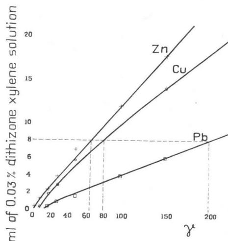
Fig. 8. The titration of standard solutions of Cu, Pb and Zn with 0.03 percent dithizone-xylene solution.
