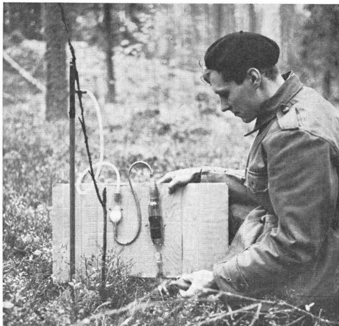
Fig. 3. The soil air pumping system.
