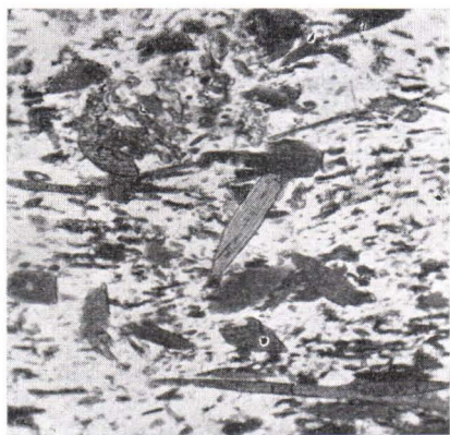
Fig. 1. Idiomorphic hornblende prisms occurring at random in the ground mass of plagioclase porphyrite. East of Lake Vaavujärvi, Orivesi. Nic. ||. Magn. 42 ×.
