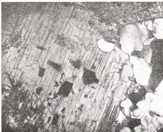
Fig. 8. Microcline antiperthite in homoaxial intergrowth with plagioclase. 12 \times . Nicols +.
