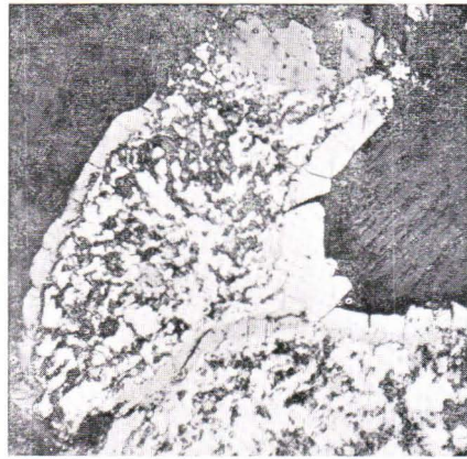
Fig. 2. Coating of chalcocite on pyrite due to peripheral replacement. Flakes of biotite at the sides. Etched (10 secs.) in concentrated \text{HNO}_3 . Ord. light. \times 290 .
