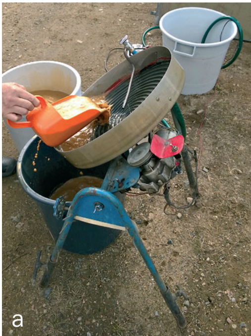
Figure 2. (a) Spiral concentrator, also called the "Gold hound". (b) Knelson separator. Photos: P. Sarala (a) and H. Koskinen (b)
