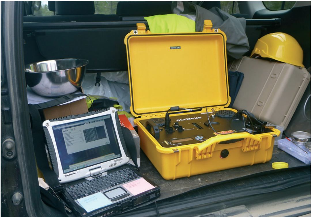
Figure 3. Olympus Terra portable XRD/XRF instrument wirelessly connected to field laptop. Photo: H. Koskinen
