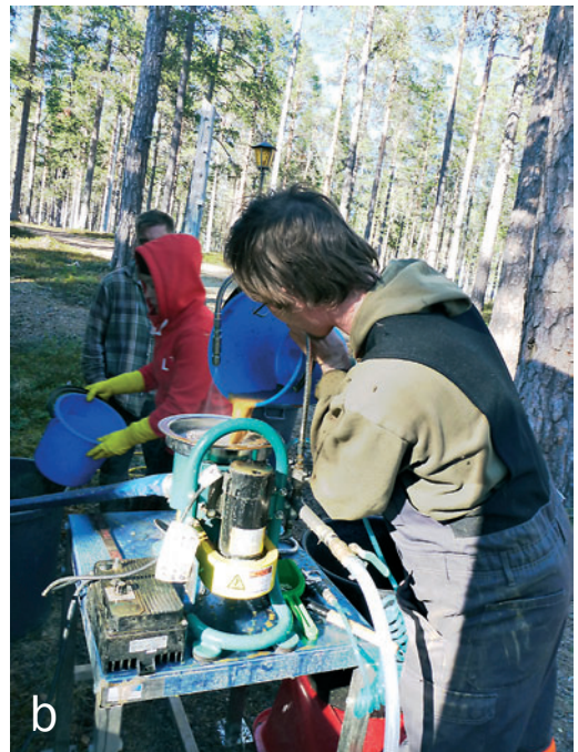
Figure 2. (a) Spiral concentrator, also called the "Gold hound". (b) Knelson separator. Photos: P. Sarala (a) and H. Koskinen (b)
